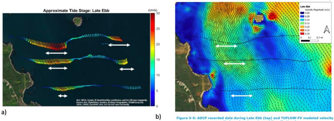
A5. During late ebb conditions, the data-model mismatch is particularly striking. None of the Tuflow transects do not represent many basic aspects of measured tidal flows along the ADCP transects. The model significantly underestimates the spatial structure and magnitude of the outflow jet along all three transect lines (white arrows).
