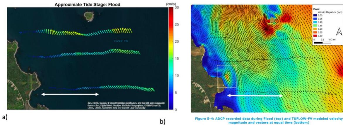
A4. At the mid-flood stage of the semi-diurnal tide, the model simulations do not appear to represent basic aspect of the observed tidal flows. The white arrow highlights how the model misses the width of the tidal stagnation zone (blue colors in the data figure (a)). The comparison also shows the data does not appear to represent a strong feature that is seen in the model (white box), or the high energy region just off the coast, north of the southern ADCP transect line.
