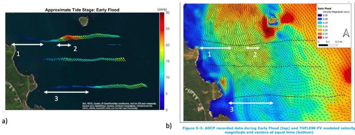
A3. The TUFLOW modeled tidal or instantaneous flows do not appear to match well with the ADCP observations. The model does not appear to capture the width of the stagnation zone (blue color arrows at sites 1 and 3), or the location of the tidal jet (site 2).
